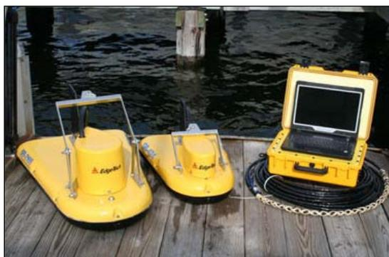
Fig. 7 - Hardware e Towfish SBP Edge Tech 3100P
